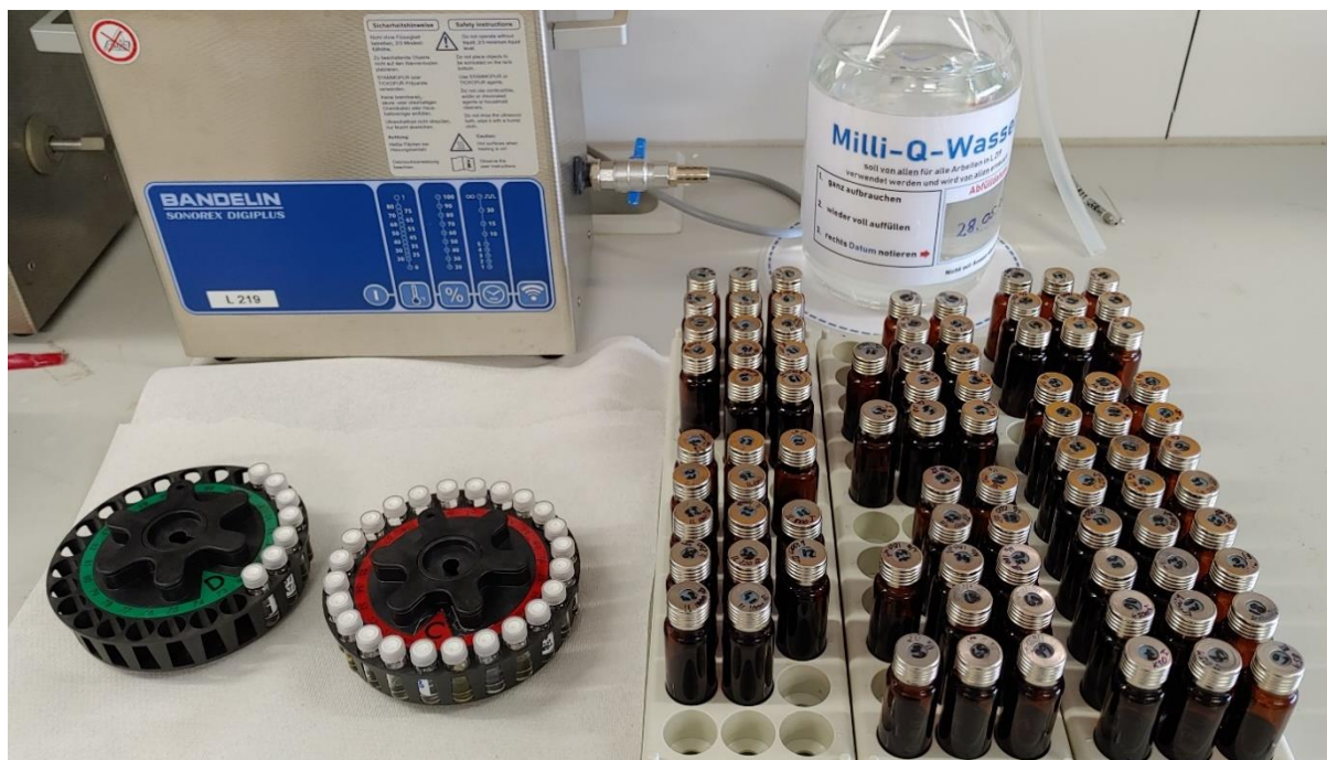
Figure 2.1 Extraction equipment as used for the ultrasonic extraction.
