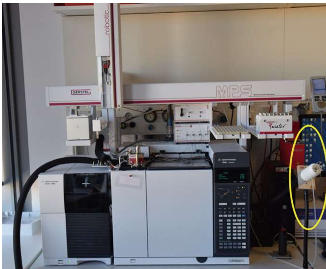
Fig. 1 GC-MS-O equipped with an autosampler and an ODP (highlighted)
