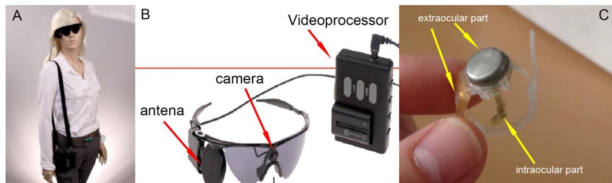
Figure 23. Argus II Retinal Prosthesis System. A – general view of the patient using Argus II Retinal Prosthesis System. B – External parts of the system including camera, antenna and videoprocessor. C - Argus II Retinal Prosthesis with depiction of its extraocular and intraocular (array) parts (Binder S, Lytvynchuk L. Argus II Retina Implantat bei an Retinopathia pigmentosa erblindeter Patientin: Ein Fallbericht. Spektrum der Augenheilkunde 2016; 30:100-5. Permission granted).
