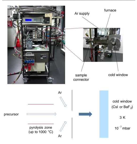
Figure 2: Top: Matrix apparatus. Bottom: Schematic representation.
