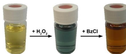
Figure 2. Reaction of 1b with hydrogen peroxide, followed by the addition of benzoyl chloride.
