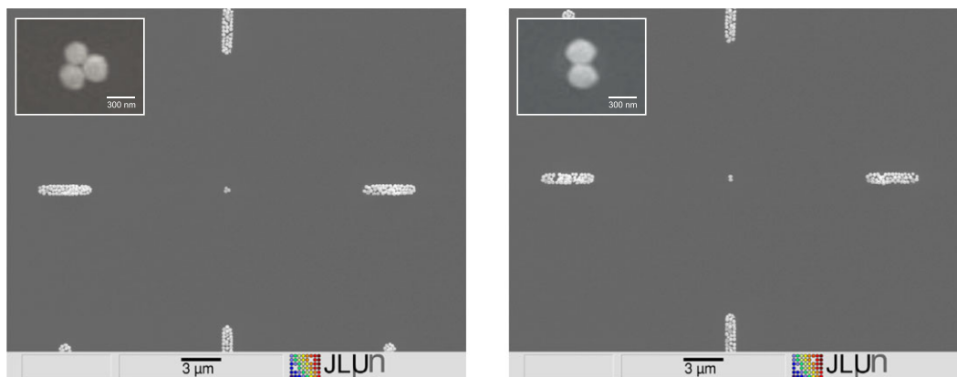
FIGURE 1 Scanning electron microscopic images of nanoparticle arrangements consisting of three (left-hand side) and two (right-hand side) 250 nm gold nanoparticles, that is, trimer and dimer. The markers surrounding the nanoparticle clusters facilitate identification of specific arrangements and their orientation during the Raman experiments [Colour figure can be viewed at wileyonlinelibrary.com ]
