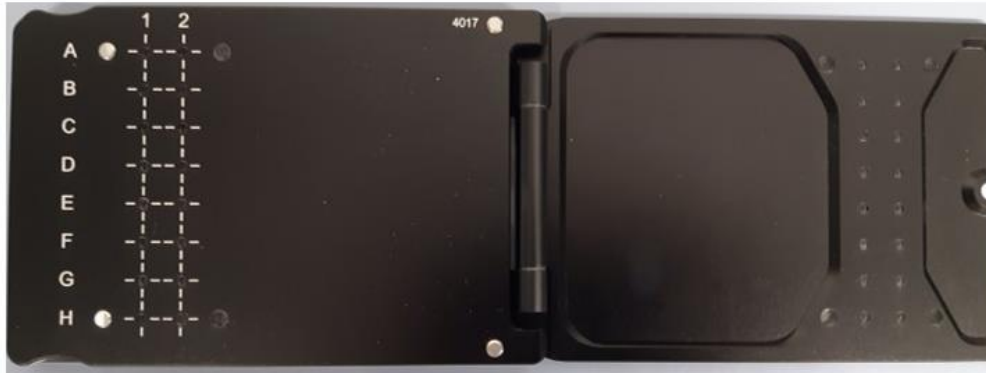
Figure B.3.5: NanoQuant Plate™. The NanoQuant™ Plate for Tecan Spark Multimode Plate Reader allows the analysis of up to 16 samples in parallel. Samples have to be pipetted on one of the 16 spots. The plate is optimized for a 2 µl sample volume.
