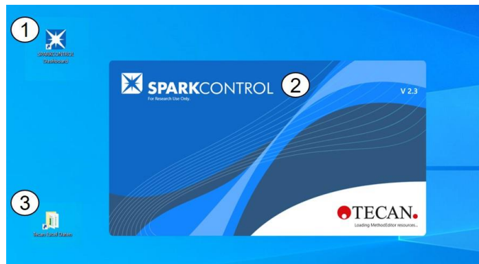
Figure B.3.2: Starting the Tecan Spark app and saving results. To start the application, click on the Tecan Spark App shortcut on the desktop (1). The program will start (2). The Shortcut for Analysis results in which the results are automatically saved as Excel sheets can be found on the desktop as well (3).
