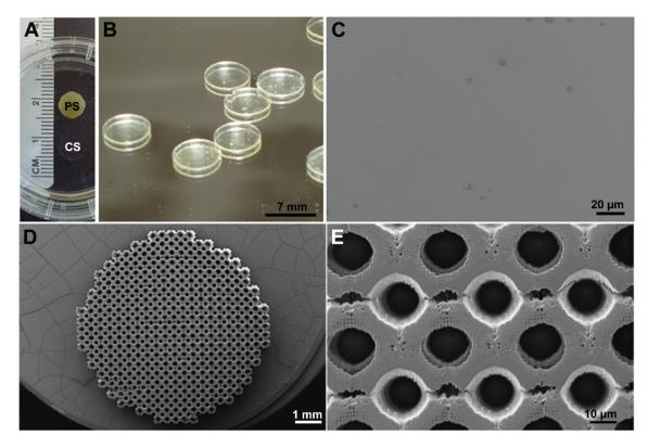
**Figure 12.** Images of porous (PS) and compact LCM scaffolds (CS). (**A**) Overview of PS compared to CS that is nearly transparent. (**B**) Higher magnification of CS. (**C**) Scanning electron microscopic (SEM) picture of the surface of CS. (**D**) SEM overview of PS. (**E**) Detail SEM of PS.
