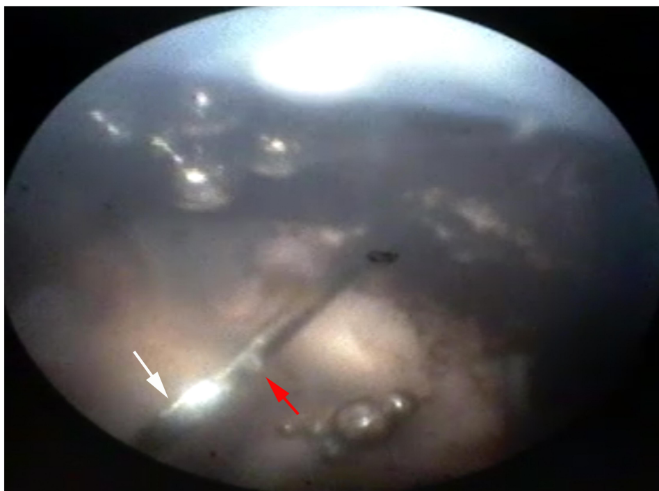
Figure 3 Enlarged view of the NDN tip after being inserted into the vitreous cavity of the cadaver pig eye (imaging performed with an E4 Ophthalmic Endoscopy System Endo Optiks®). Light reflection depicts closed front opening (white arrow). Red arrow indicates side port of the NDN. (Created by L. Lytvynchuk.)
