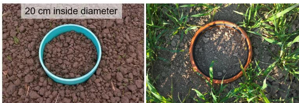
Figure 9: Chamber-collar offset settlement for soil CO 2 efflux measurement, LTE-BNF (photo: Yavar Vaziritabar).
