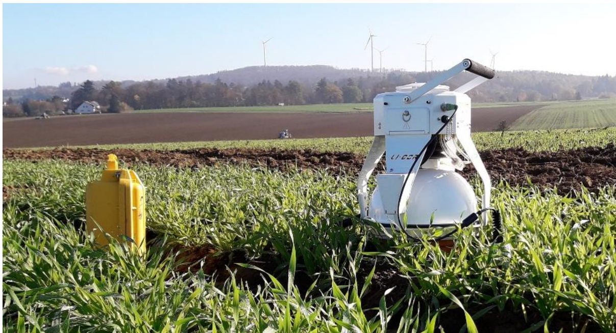
Figure 8: Soil CO 2 efflux measurement by Licor-870 CO 2 /H 2 O infrared gas analyser-IRGA (SSA-1005) in LTE (photo: Yavar Vaziritabar).
