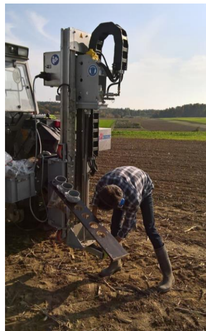
Figure 4 (left): Soil sampling techniques, steel auger for drilling and taking soil sample (Photo: Yavar Vaziritabar). Figure 5 (right): Sampling device (Multiprob 120-UP)-Nietfeld company, Experimental station “Weilburger Grenze” Giessen (Photo: Markus Kolmer).
