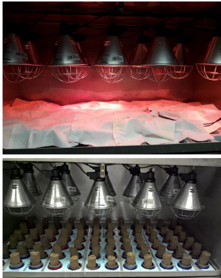
Figure 7: Drying chamber and sampling method to extract soil arthropods, high gradient technique, LTE-BNF (photo: Yavar Vaziritabar).
