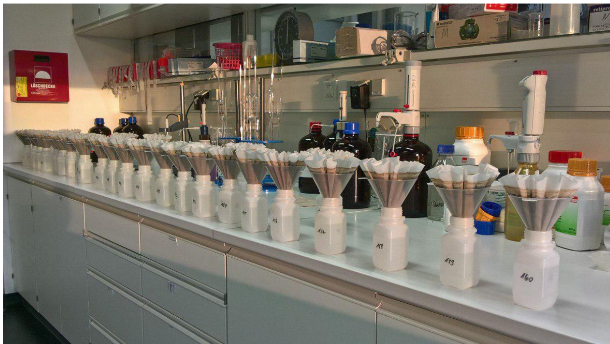
Figure 6: Soil extraction and filtration method for nitrate ( \text{NO}_3^- ) N analysis, laboratory of the department of Agronomy (photo: Yavar Vaziritabar).
