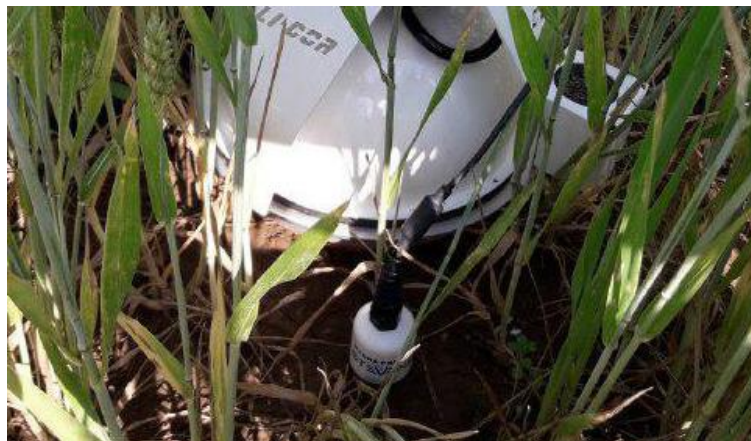
Figure 10: The Stevens HydraProbe soil sensor (photo: Yavar Vaziritabar).
