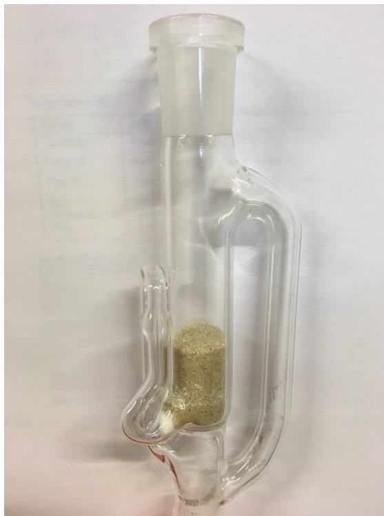
Figure 2 In situ formation of the OXB catalyst via condensation through a micro Soxhlet filled with CaH 2 and sand.
