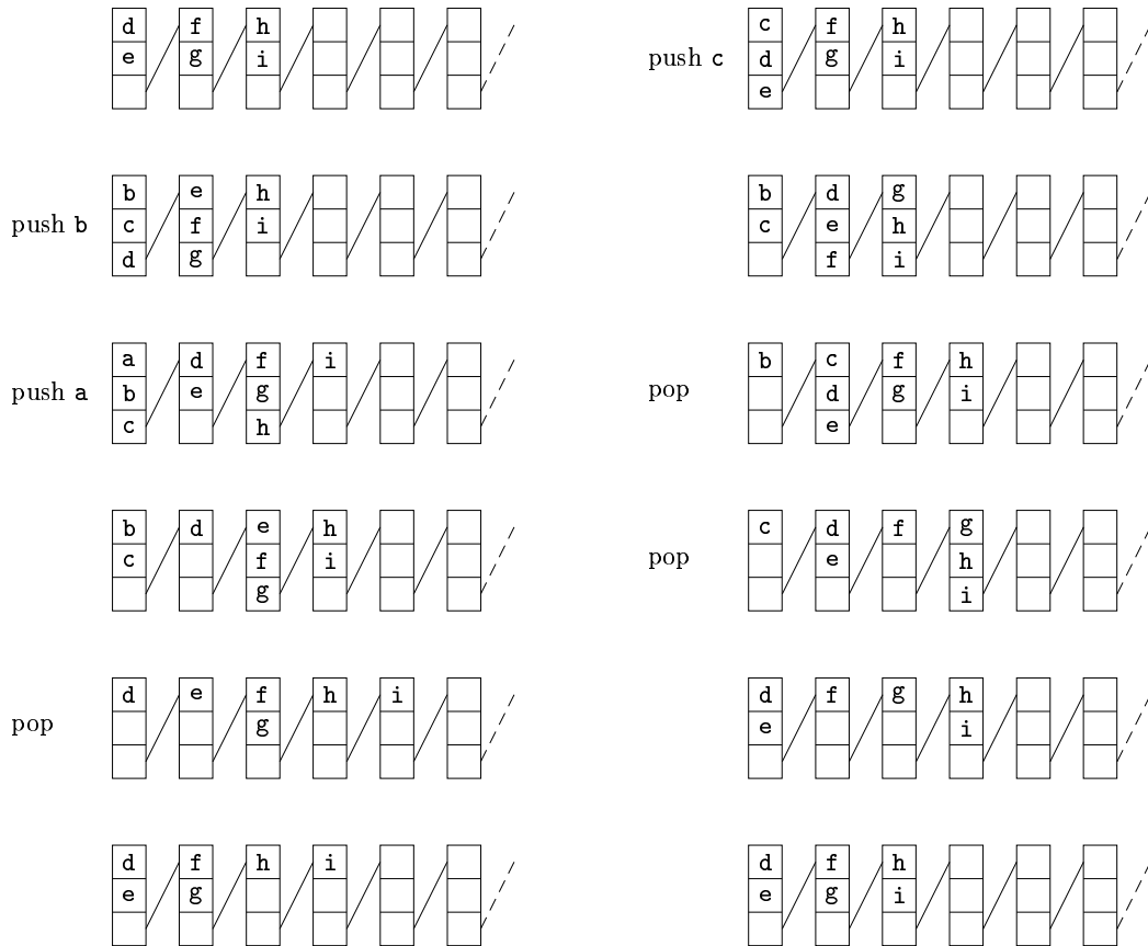
Figure 5: Example for pushdown store simulation by a two-way device.
