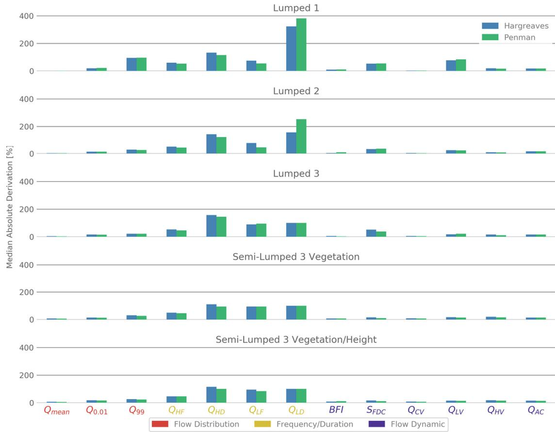
**Figure 1.7:** Median absolute deviations (%) of simulated versus observed hydrological signatures. Smaller values indicate smaller error in the simulation.
