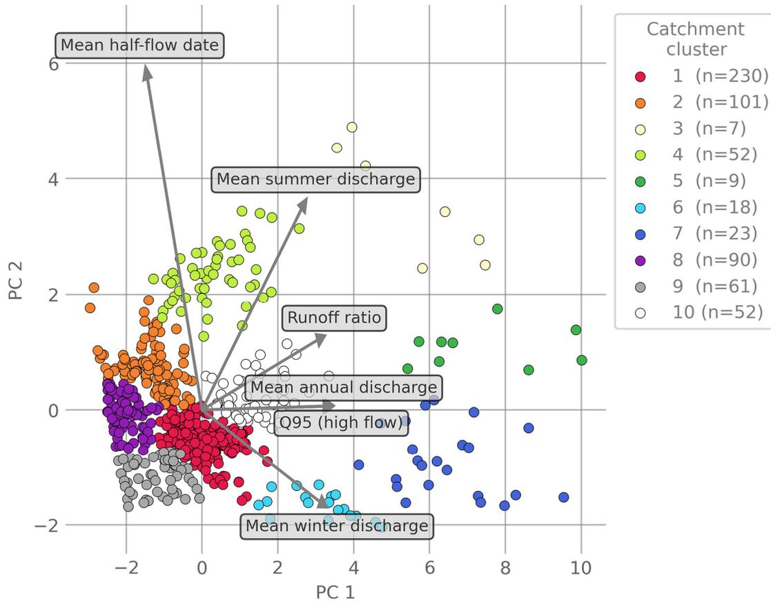
**Figure II.3:** Biplot of the principal components (PCs). Colors indicate the cluster of the catchment. Grey arrows indicate the loadings of the original catchment attributes in the PCA space.
