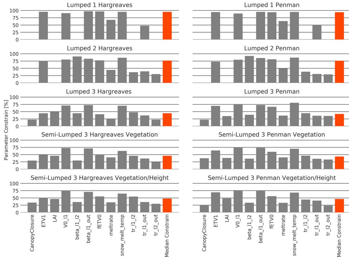
**Figure 1.5:** Parameter constrainability for all model structures separated by parameters. Red bar marks the median parameter constrainability for each model. Larger bars indicate larger constrained parameters. Parameter constrainability is defined as the difference
