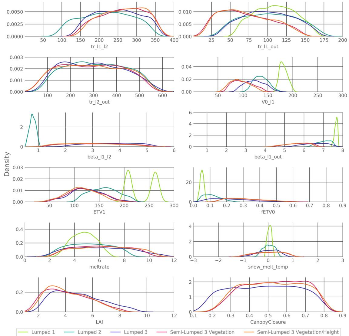
**Figure I.4:** Posterior parameter distribution separated by model structures shown in different coloured lines. Different PET calculations for a model structure are pooled. X-axes scales equal the a priori distribution of the parameters before calibration. Lines are fitted with a Gaussian kernel density function.
