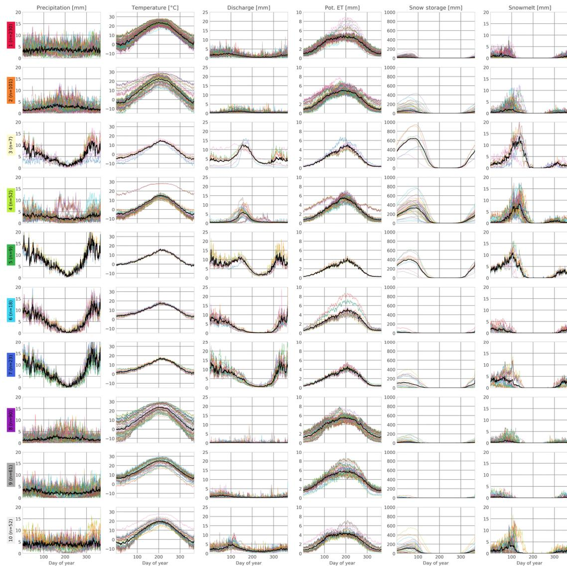
**Figure II.6:** Meteorological attributes of the clustered CAMELS catchments averaged by day of the year. Potential evapotranspiration (Pot. ET) was calculated with Hargreaves–Samani (Samani, 2000). Snow storage and melting was calculated using a temperature-based approach described in
