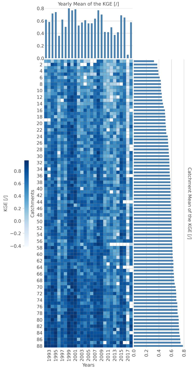
**Figure III. 5:** Heatmap of the Kling-Gupta Efficiency (KGE) (measure of catchment complexity) for the 88 catchments of the Hesse dataset, separated by years. Darker colors indicate lower complexity. Bar charts depict the mean values for the rows and columns.
