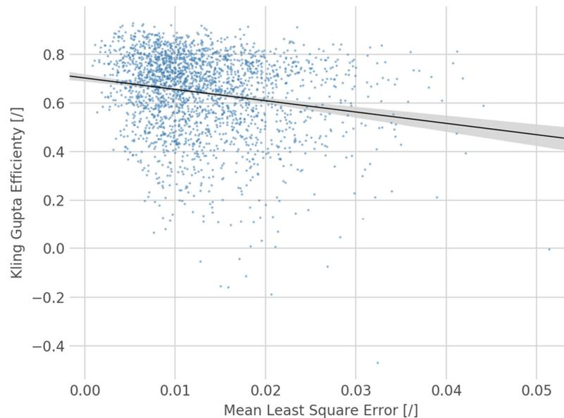
**Figure 8:** Relationship between the model efficiency of the HYMOD Model (measured with the Kling-Gupta Efficiency) and the catchment complexity (measured with the Mean Least Square Error). The trend of the regression is significant with  $p$ -value  $< 0.001$
