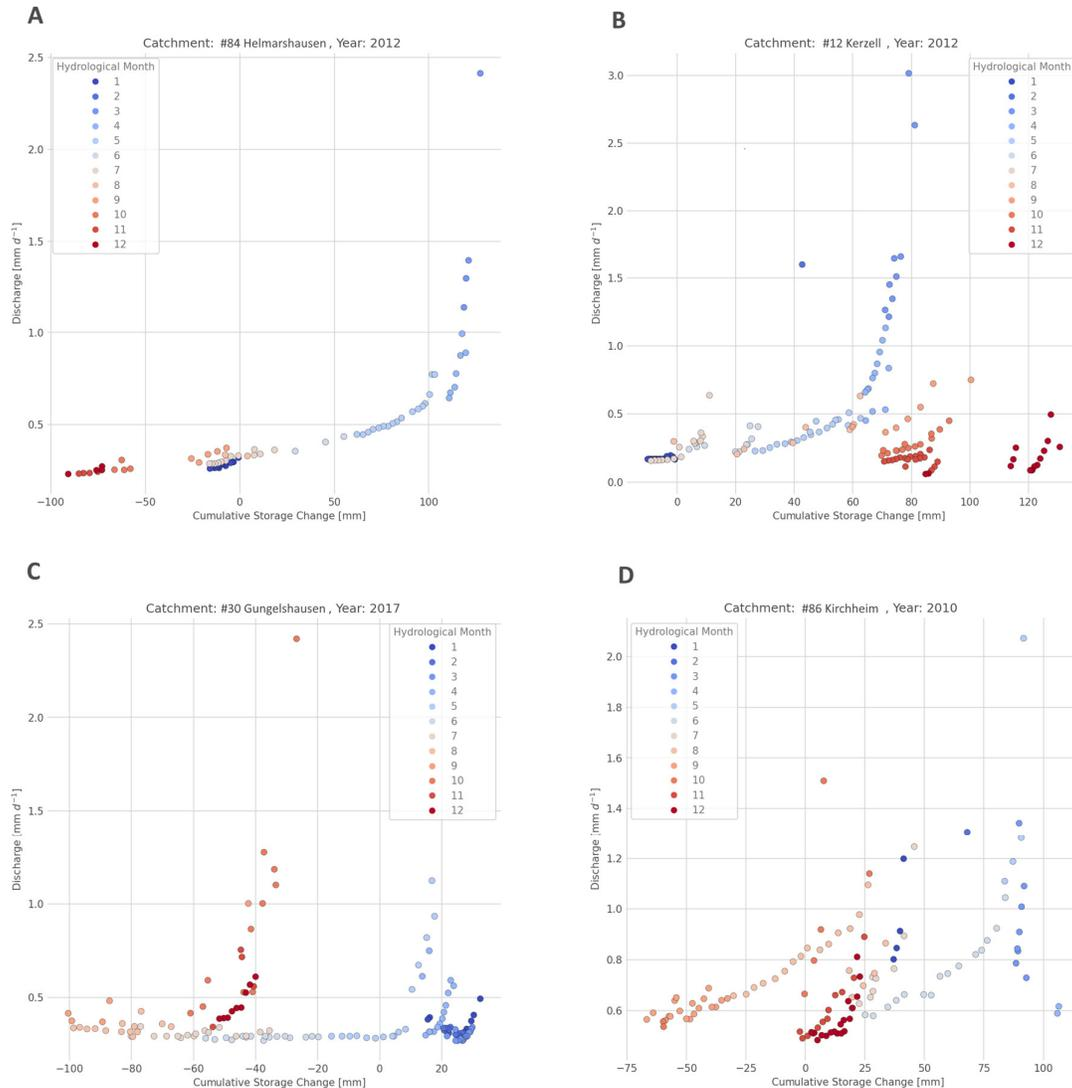
**Figure III.4:** Plots show cumulative change in storage against discharge during recession periods in a hydrological year. Color indicates the month of the hydrological year. Examples of the patterns in the storage-discharge relationship. A) an almost perfectly exponential storage-discharge relationship B) low discharge, even though the storage is higher than at previous peak discharge C) peak discharge, even though the storage is lower than at previous peak discharge D) erratic behavior.
