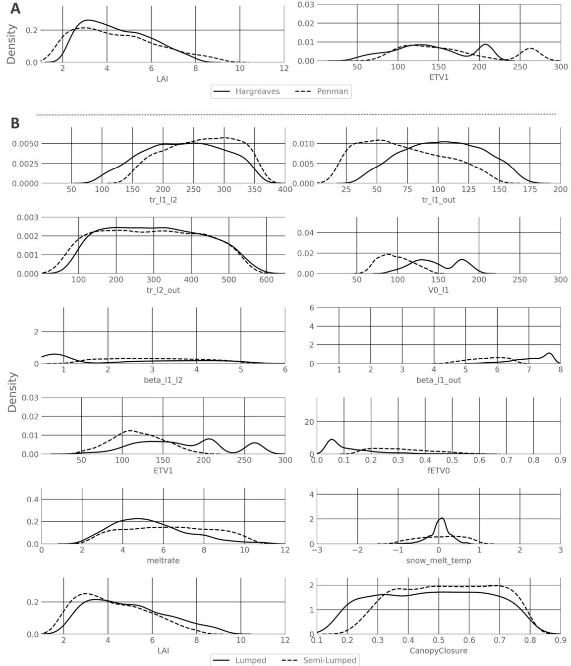
**Figure 1.6:** Posterior parameter distributions separated by PET method for the parameters influenced by PET method. Different model complexities are pooled (A). And distributions separated by spatial subdivision for the parameters influenced by spatial subdivision.
