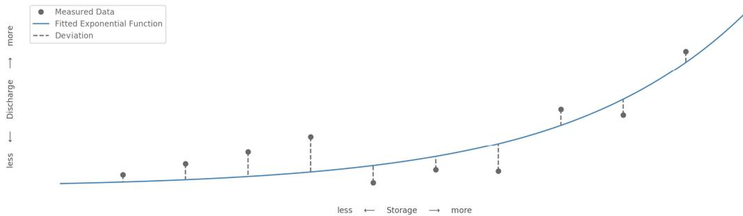
**Figure III.3:** Visualization of the deviation of the measured and the idealized storage-discharge relationship (artificial data).
