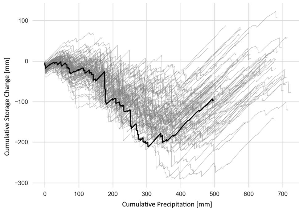
**Figure 7:** Cumulative precipitation plotted versus cumulative storage change for all catchments in the Hesse dataset for the year 2018. Grey lines are the single catchments. Black line is the median of all catchments.
