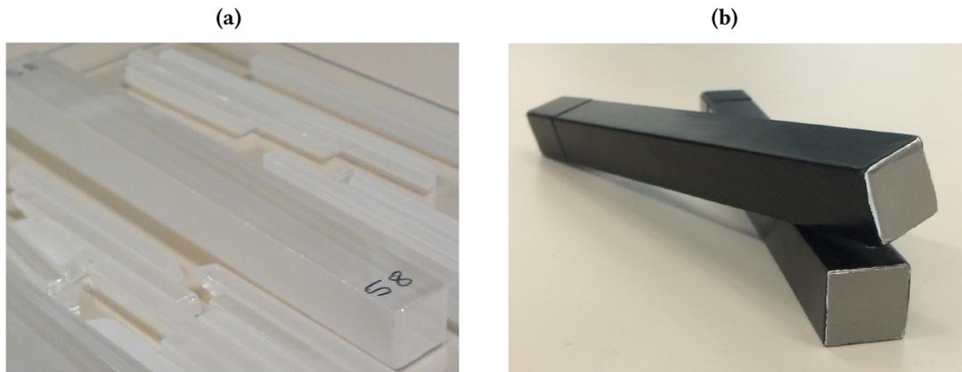
**Fig. 4.7.:** (a) A prototype  $\bar{\text{P}}\text{ANDA}$  EMC crystal cut into several smaller crystals. As can be seen, the smaller crystals easily break, therefore a bigger one (b) has been chosen for the prototype detector .
