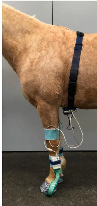
**Figure 1.** Horse equipped with the Hoof™ System.
