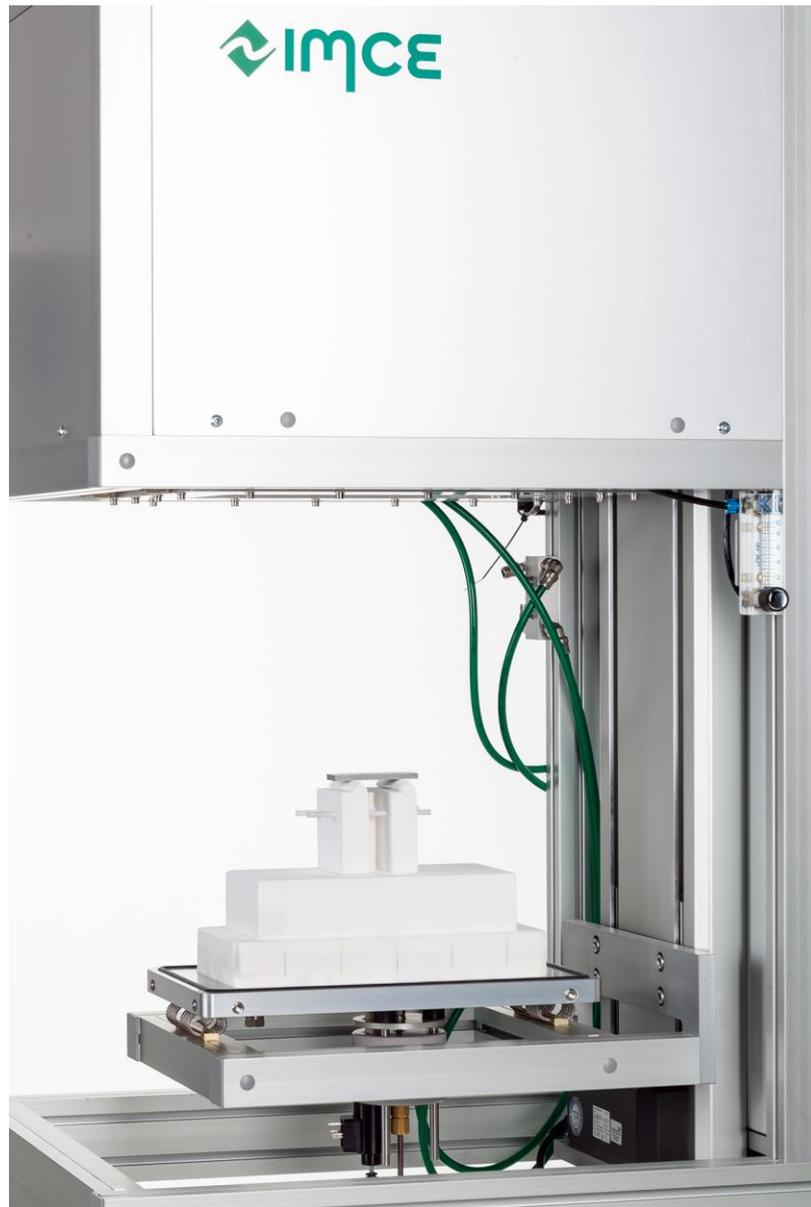
**Figure 4-7** High temperature setup for the IET
