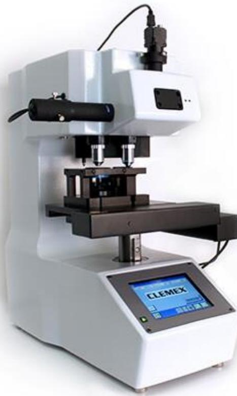
*Figure 4–5 Clemex hardness testing machine*
