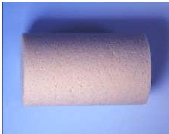
**Abb. 16:** Polyurethanschaumzylinder 50mm x 30mm
