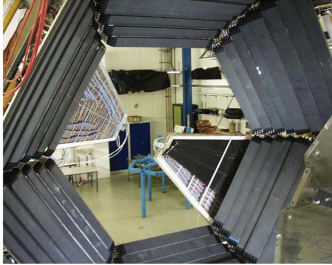
Figure 2.7: Photo of the HADES TOF detector before its installation. In the central part of the photo two sectors of the Pre-Shower detector [128] can be seen. The Pre-Shower detector was replaced by an electromagnetic calorimeter in the  $AgAg$  data run.
