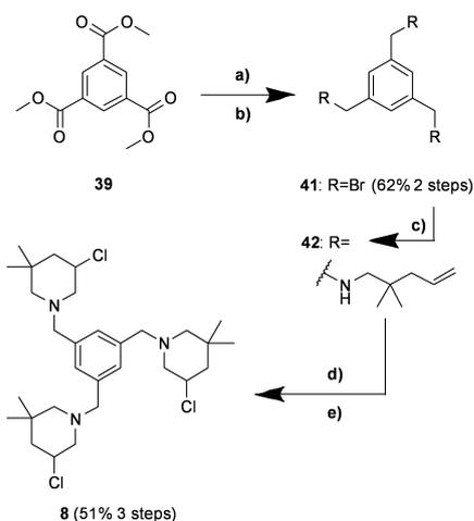
**Scheme 2.** Synthesis of *tris*-3-chloropiperidine **8**. a) LAH, dry THF, 0 °C to RT to reflux, 18 h; b) PBr<sub>3</sub>, dry Et<sub>2</sub>O, 0 °C to RT, 24 h; c) 2,2-dimethylpent-4-en-1-amine **12**, dry CH<sub>2</sub>Cl<sub>2</sub>, 0 °C to RT, 68 h; d) NCS, dry CH<sub>2</sub>Cl<sub>2</sub>, 0 °C to RT, 2.5 h; e) TBAI (cat.), dry CHCl<sub>3</sub>, reflux, 4 h.
