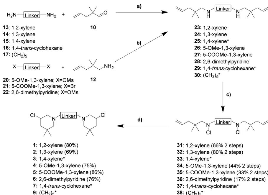
**Scheme 1.** Synthesis of *bis*-3-chloropiperidines 1–6. a) NaBH(OAc)<sub>3</sub>, AcOH, dry CH<sub>2</sub>Cl<sub>2</sub>, 0 °C to RT, 16–18 h; b) NaH, dry THF, 0 °C to RT, 20–22 h; c) NCS, dry CH<sub>2</sub>Cl<sub>2</sub>, 0 °C to RT, 2.5–3 h; d) TBAI (cat.), dry CHCl<sub>3</sub>, 60 °C (oil bath temperature), 2–2.5 h (inseparable diastereomeric mixture). \*The synthesis of compounds 3, 7 and 9 as well as their corresponding precursors has been described elsewhere.<sup>[4b]</sup>
