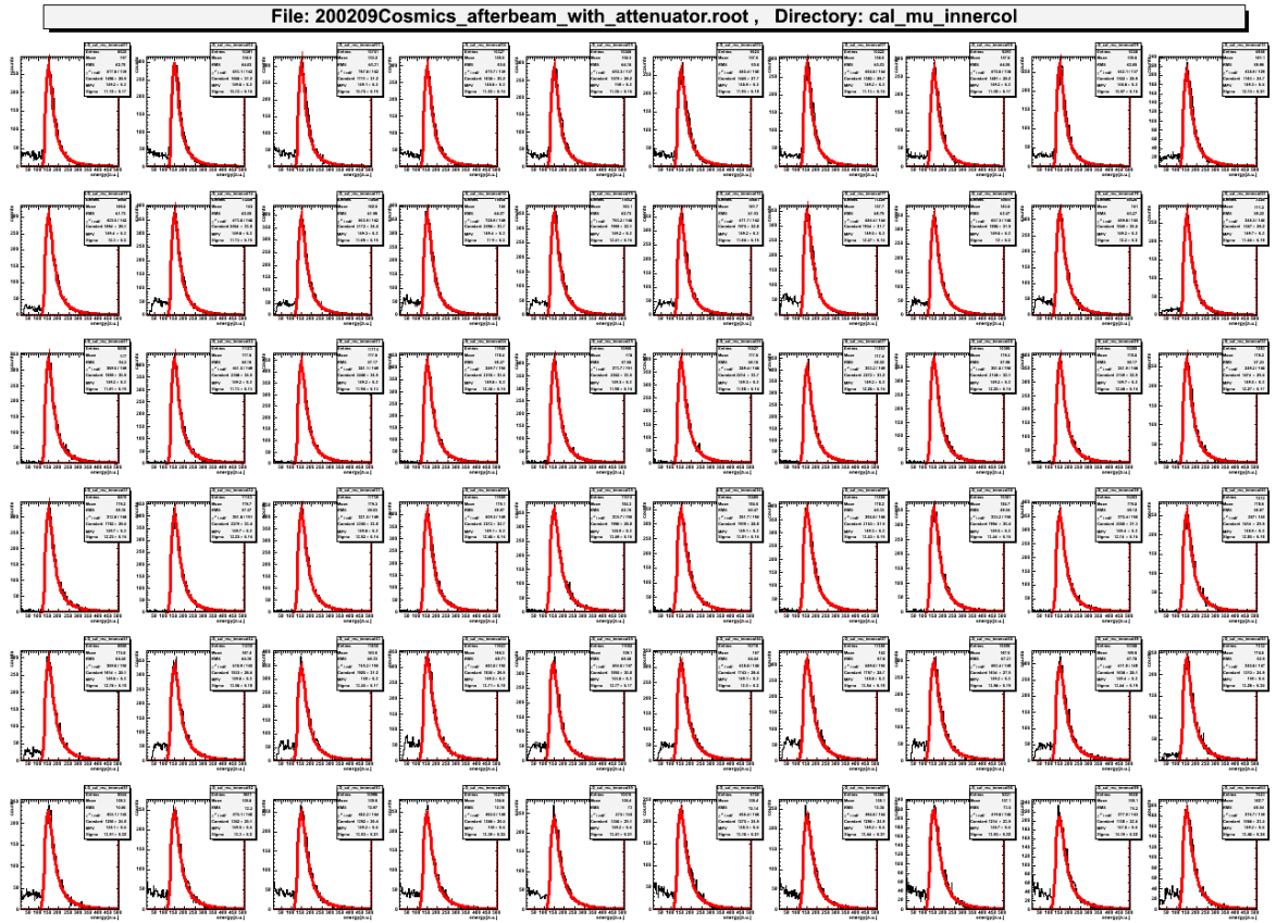
Figure 5.19: Calibrated cosmic radiation data with the column cut condition. A fit with a Landau distribution (red) is applied in order to verify the alignment.
