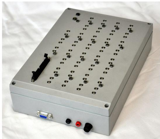
Figure 4.8: Picture of the TTL trigger system. Its interface consists of 64 TTL outputs (32 individual channels) and a monitor output [Jesch, 2016].
