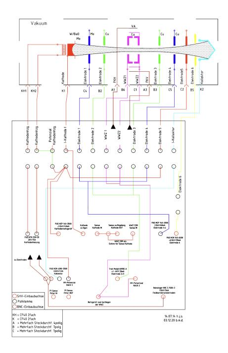
${\bf Abbildung} \ {\bf C.1} - {\bf Anschluss-} \ {\bf und} \ {\bf Verteilerplatte} \ {\bf f\"{u}r} \ {\bf Elektronenkanone} \ {\bf mit} \ {\bf Ansteuerung} \ {\bf und} \ {\bf Scansystem}.$
