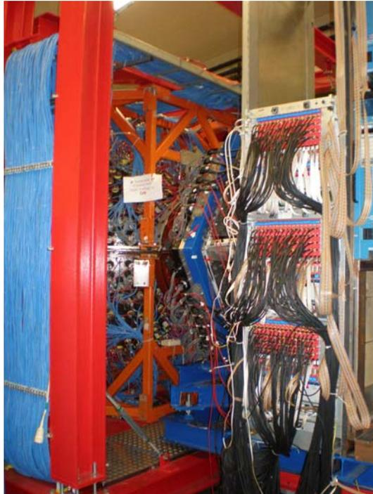
**Figure 3.1:** On the left side the Crystal Ball on its platform, on the right side the TAPS detector with its readout electronics is shown. TAPS is mounted on rails, so it can be moved easily close to the Crystal Ball for measurements.
