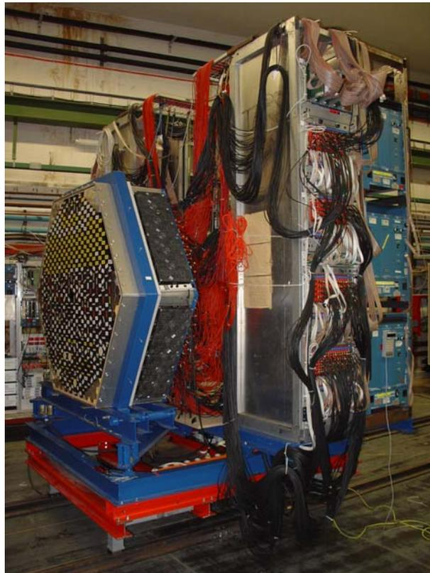
**Figure 3.7:** Photograph of the TAPS detector system. The readout electronics is mounted on the TAPS frame on both sides of the forward wall. The electronics for 4 blocks, together with the high voltage supplies are shown.
