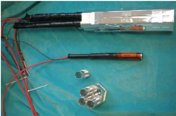
(a) A complete module consisting of 4  $\text{PbWO}_4$  crystals. In front a single PMT is shown and the main housing block for the PMTs for coupling to the crystals.
