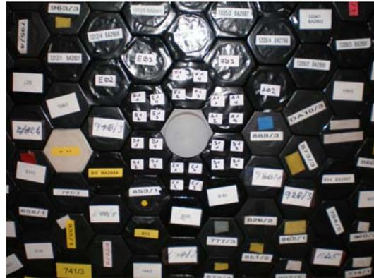
(b) 24  $\text{PbWO}_4$  crystals as the inner ring, mounted in the TAPS forward wall.
