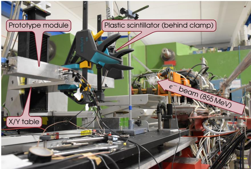
**Figure 4.13:** Setup of the prototype beam test. The electron beam enters from the right-hand side. Before it hits the module head on, it passes through a thin plastic scintillator paddle. The module was clamped to a remotely controllable table allowing movements in  $x$  (horizontal) and  $y$  (vertical) directions. The large green structure in the background is one of the two 450 t heavy dipole magnets of RTM<sub>3</sub>.
