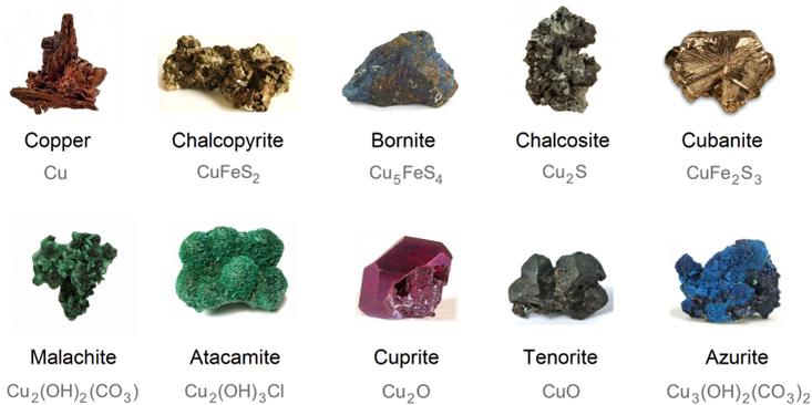
Figure 1.1.: Overview of the most common copper ores. [2]
