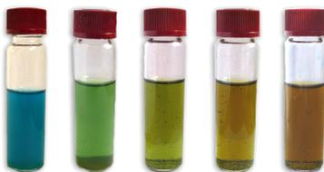
Figure 2.16.: Color change of cluster I in denatured ethanol: The solution turned from blue to red-brown within a day. The olive colored solid disappeared and cluster II could be obtained as emerald green crystals.
