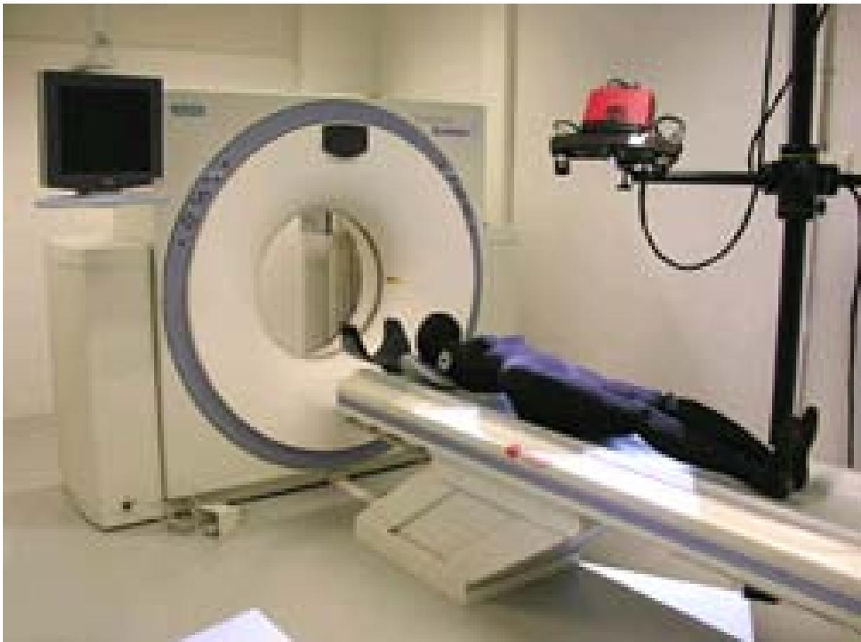
Abb. 2: MSCT Emotion 6 (Siemens, Germany) & ATOS III (GOM, Germany). Simulation of 3D surface scanning with a puppet (<http://www.virtopsy.com>)
