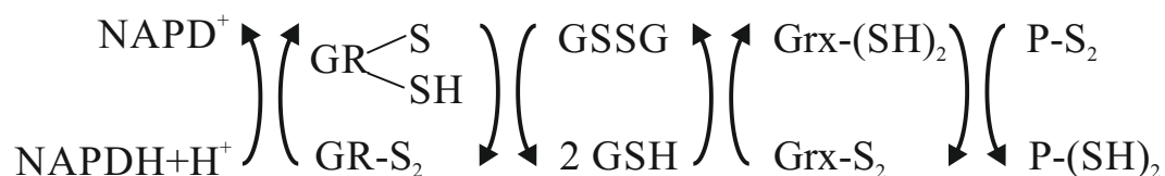
Figure 1.5: The dithiol mechanism of Grx.
