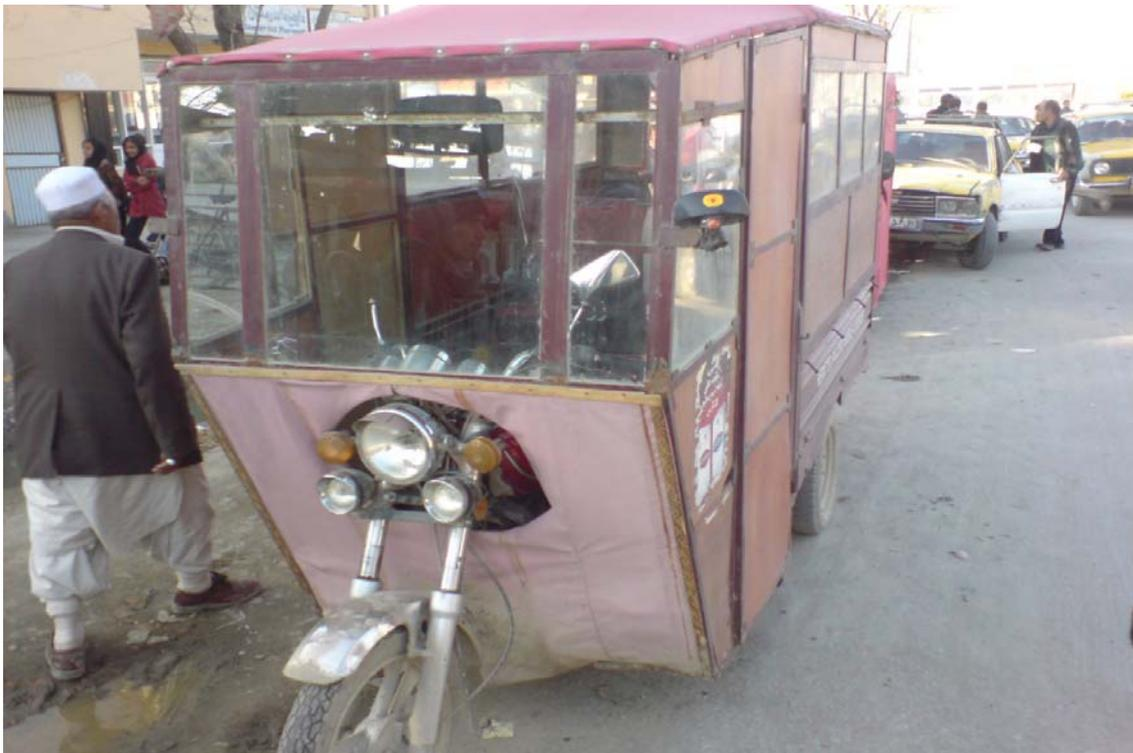
**Photo 3.4: Three wheeled motorcycles turned to the auto rickshaw form for transferring passengers (Source: photo: NOORI 2008).**
