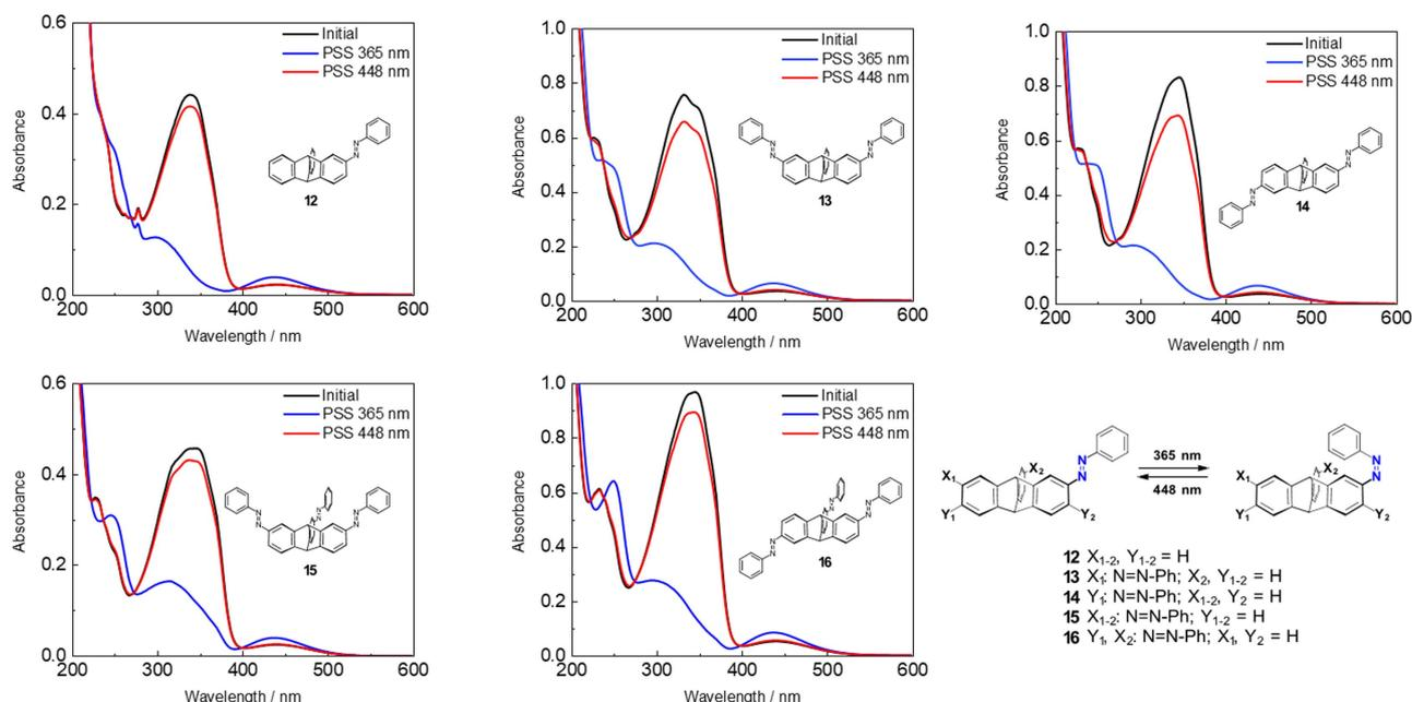
**Scheme 2.** UV-Vis spectroscopy of (*meta*)-TrpABs **12–16** in acetonitrile/H<sub>2</sub>O (90:10) at a concentration of  $2 \times 10^{-5} \text{ mol L}^{-1}$ . The solutions were irradiated with light of 365 nm (purple) and subsequently with light of 448 nm (blue) until the PSS was reached.
