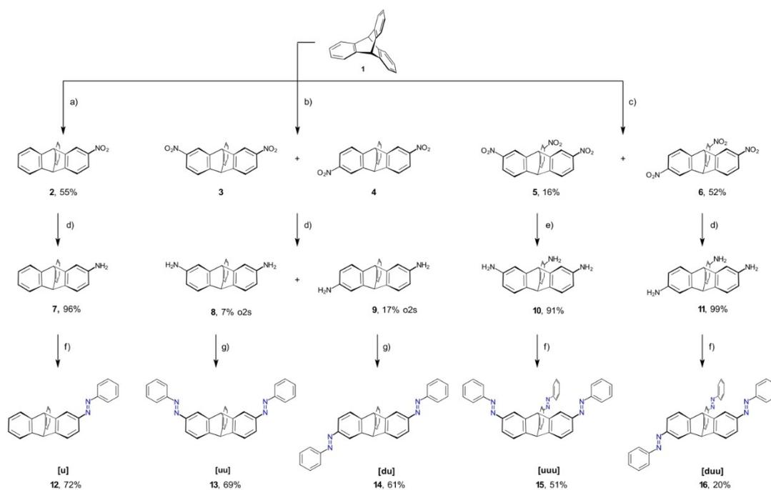
Scheme 1. Synthesis route towards *meta*-TrpABs **12–16**. a) conc.  $\text{HNO}_3$ , 75 °C, 24 h; b)  $\text{KNO}_3$ , TFAA, ACN, RT, 24 h; c) fuming  $\text{HNO}_3$ , AcOH, 0 °C, 1 h; d)  $\text{H}_2$ , Pd/C, MeOH, overnight; e)  $\text{H}_2$ , Pd/C, MeOH, 2 h; f) nitrosobenzene, AcOH, toluene, 60 °C, 24 h; g) nitrosobenzene, AcOH, toluene, 60 °C, 48 h. o2s: over two steps.
