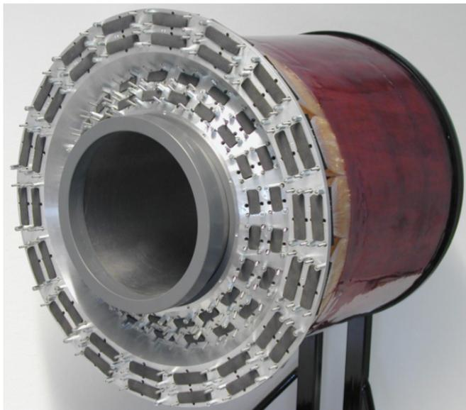
Figure 4.2.4: [46] Picture of the assembled SFT mounted over a mockup scattering chamber.
