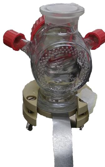
FIGURE 3.5: One WE chamber is shown, prepared for LbL-coating. The ITO electrode and graphite paper were mounted to the glass body and coating solution was added through the second flange. During incubation the flange was covered with parafilm. Reactors were incubated shaking in this upright position.
