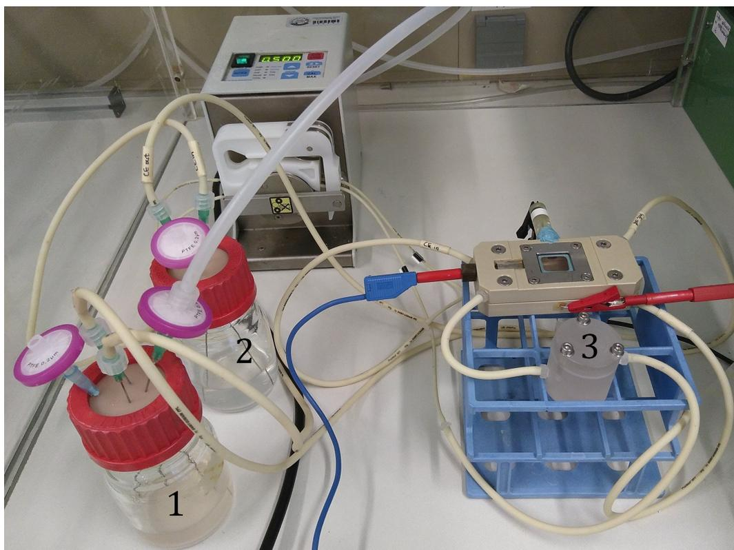
FIGURE 3.10: The experimental set-up of the flow cell in the incubator hood (without the CLSM) is shown. Component 1 is the WE reservoir, 2 the CE reservoir and 3 the bubble trap.
