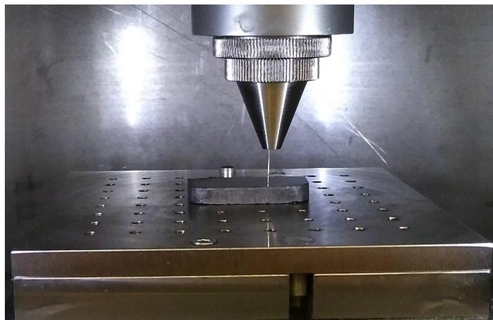
FIGURE 3.6: A sample in the HR-SKP chamber with the tip positioned few  $\mu\text{m}$  above the measured surface.
