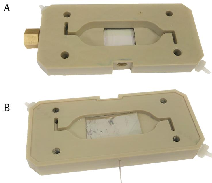
FIGURE 3.9: The two chambers of the flow cell are shown; with (A) the WE with the transparent ITO anode atop the chamber and (B) the CE chamber with the platinum cathode.
