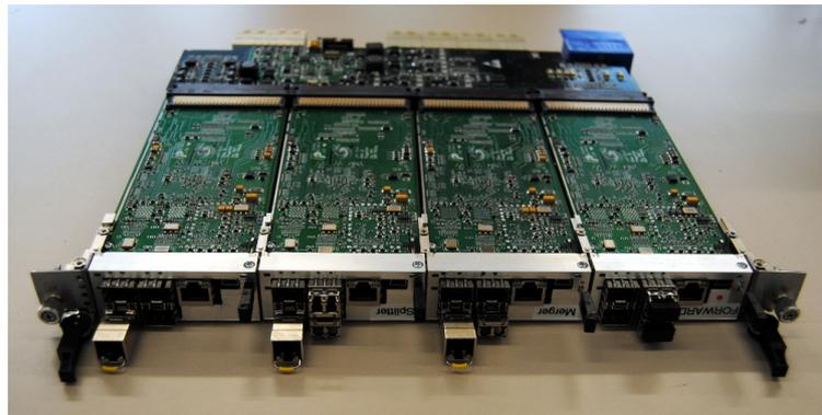
**Figure 3.2.:** Prototype of AdvancedTCA carrier board equipped with 4 xFP. [59]
