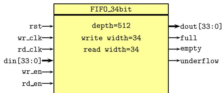
**Figure B.22.:** Diagram of the FIFO\_34bit ports.
