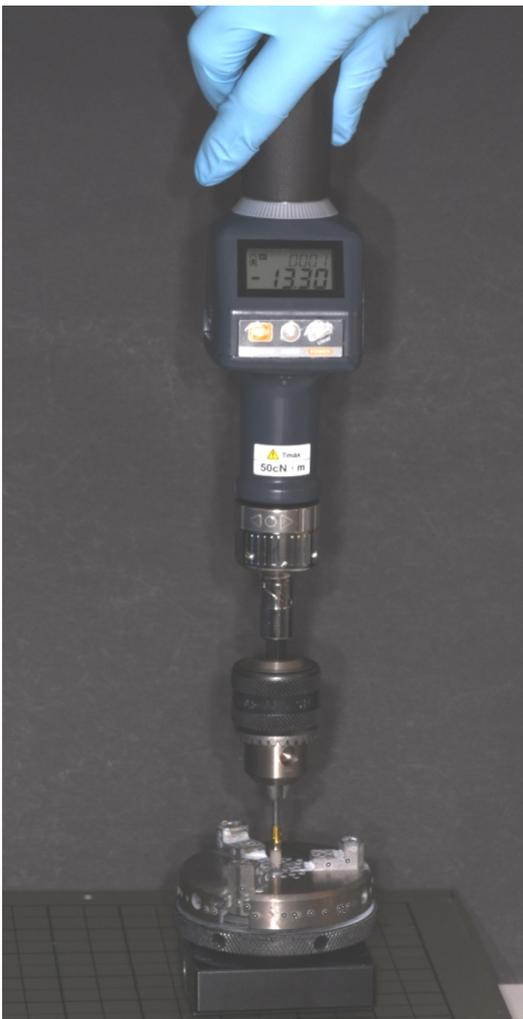
fig. 32) Unfastening the implant-abutment connection
