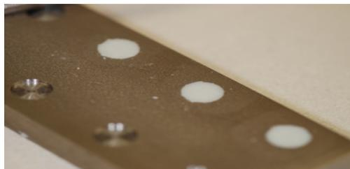
fig. 19) Specimens after excess removal
