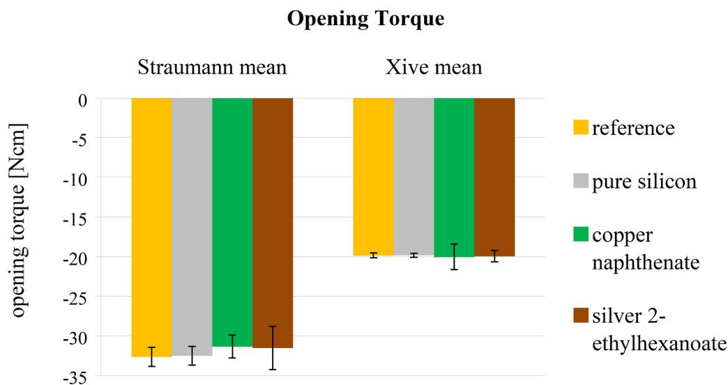
fig. 57) Comparison of means (with standard deviation) of opening torque.
