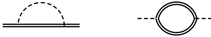
Figure 3.3: Diagrams that yield complex contributions to the time-ordered and retarded quark self-energies and RPA meson polarizations.
