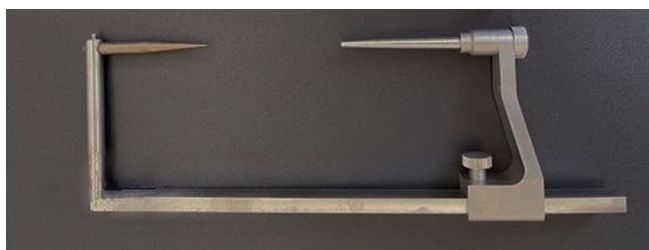
FIGURE 2 Modified aiming device (AD), with two exchangeable adapters: First for pin insertion, 1.6 mm inner diameter, second for inserting the cannulated drill bit, inner diameter 2.75 mm.
